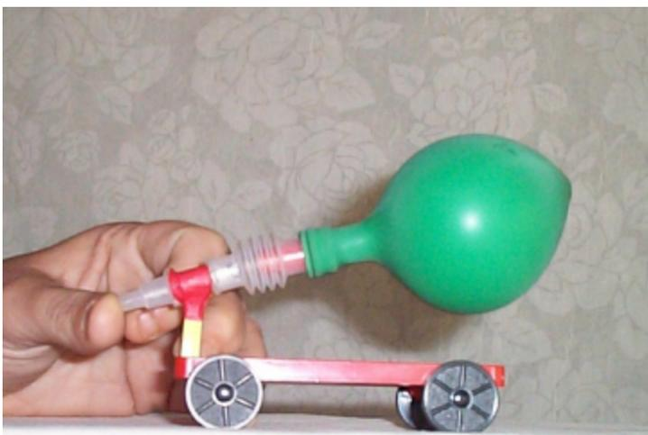
blow up the balloon that is attached to the car, place the care on the floor, and release the car. As the gas is released from the balloon, the car goes in the opposite direction.
